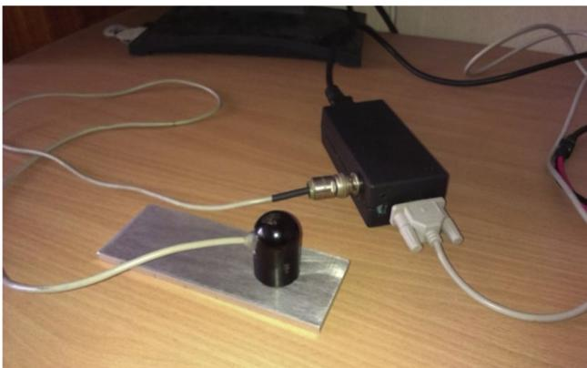
Fig. 4. Exterior view of the measuring unit of eddy current measuring system.
