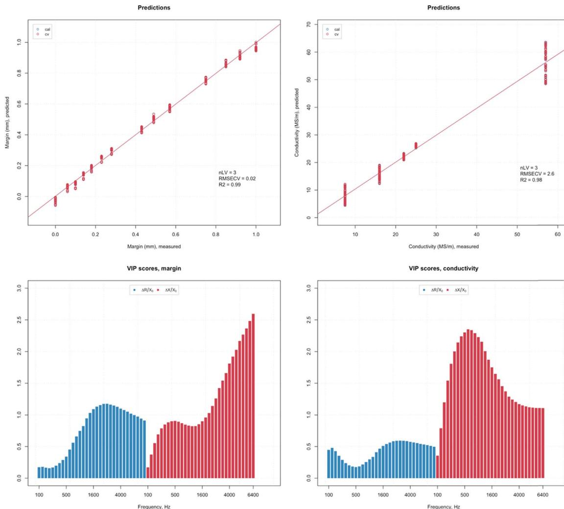
Fig. 5. Predicted vs. measured plots (top) and VIP-scores (bottom) for the PLS regression models.
