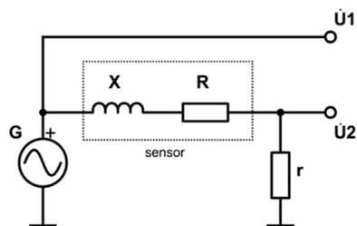
Fig. 1. A schematic diagram of the measurement system.
