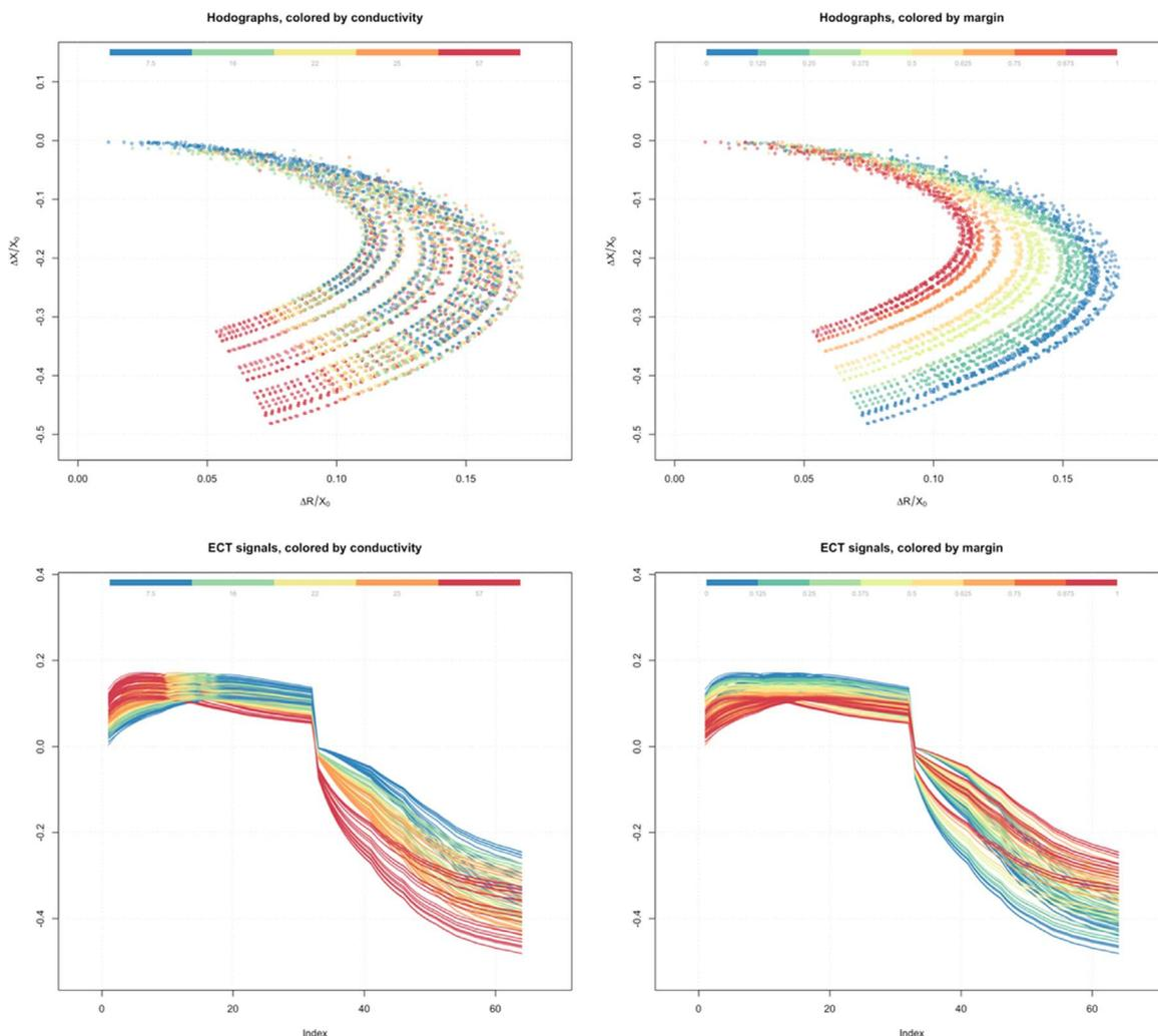
Fig. 2. Representation of measured relative reactance and resistance in form of hodographs (top) and line plots (bottom).
