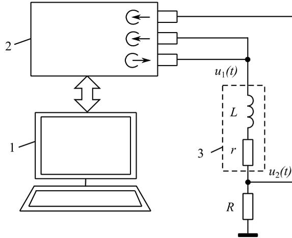
**Figure 1.** A simplified scheme of the automated measuring and computing complex for multifrequency eddy current testing.
