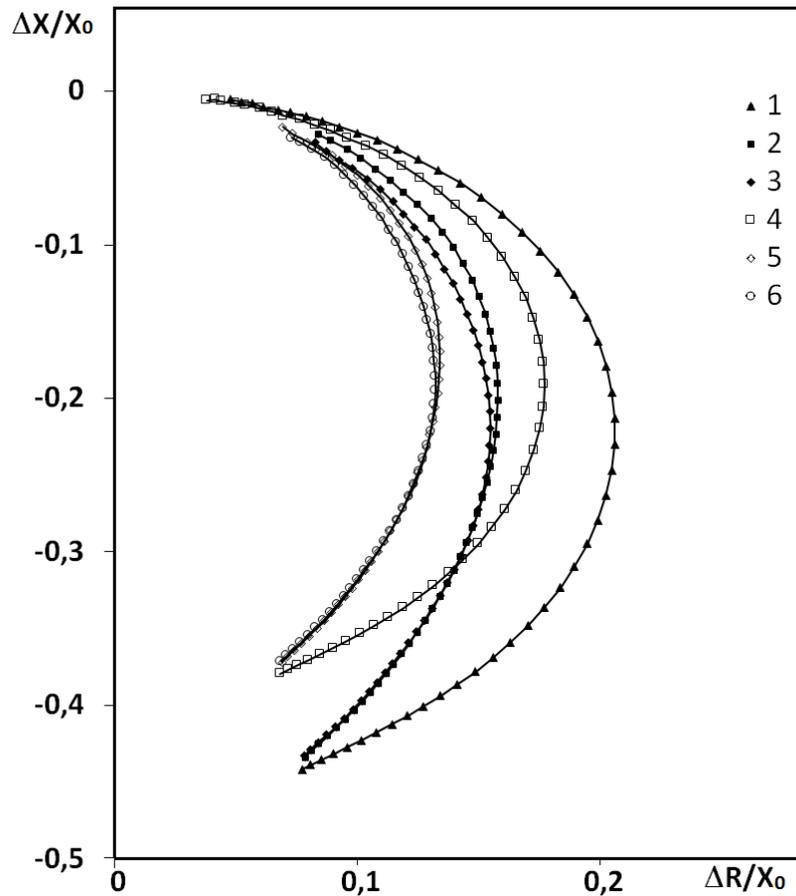
**FIGURE 2.** Experimental hodographs for aluminum samples of various thicknesses with applied dielectric layer. Dielectric layer thickness  $s = 0.6$  mm, plate thickness  $h$ : 1 – 1.43 mm, 2 – 5.72 mm, 3 – 8.61 mm;  $s = 0.2$  mm,  $h$ : 4 – 1.43 mm, 5 – 5.72 mm, 6 – 8.61 mm.
