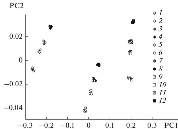
**Fig. 2.** Projections of eddy-current measurement results onto the plane of the first principal components. The gap values are for copper (1) 0.07, (2) 0.20, (3) 0.50, (4) 1.0; for manganese (5) 0.07, (6) 0.2, (7) 0.50, (8) 1.0; and for bronze (9) 0.07, (10) 0.20, (11) 0.50, (12) 1.0 mm.
