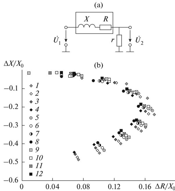
**Fig. 1.** Eddy-current measurements for copper, manganese, and bronze: (a) scheme of eddy-current measurements; (b) experimental hodographs for “sensor-sample” system. The gap values  $h$  are for copper (1) 0.07, (2) 0.10, (3) 0.14, (4) 0.20; for manganese (5) 0.07, (6) 0.10, (7) 0.14, (8) 0.20; and for bronze (9) 0.07, (10) 0.1, (11) 0.14, (12) 0.20 mm.
