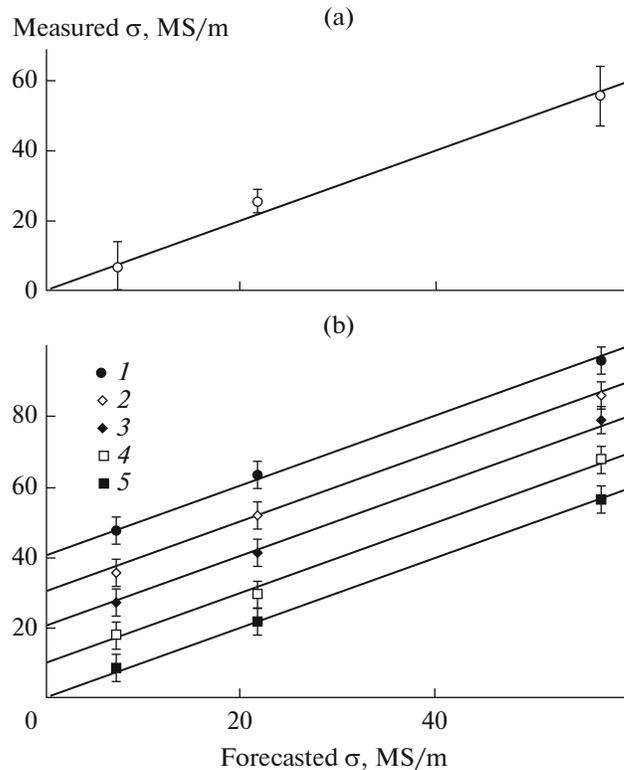
**Fig. 4.** Determining electrical conductivity: (a) gap value from 0 to 1 mm; (b) gap values ( $l$ ) from 0 to 0.2 (forecasted value  $\sigma + 40$  MS/m), (2) from 0.2 to 0.4 ( $\sigma + 30$  MS/m), (3) from 0.4 to 0.6 ( $\sigma + 20$  MS/m), (4) from 0.6 to 0.8 ( $\sigma + 10$  MS/m), (5) from 0.8 to 1.0 mm.
