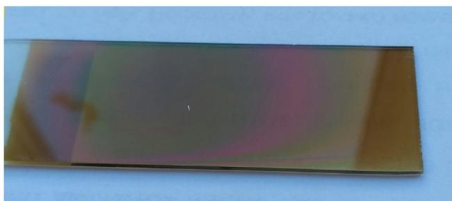
**Fig. 1.** A diamond-like amorphous carbon film deposited on the silicate glass substrate obtained by laser evaporation of carbon target. The dimension of the area covered with film is  $75 \times 25 \text{ mm}^2$ .
