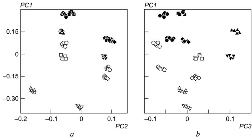
Fig. 3. Projections of the results of eddy current measurements on the plane of the first principal components  $PC1-PC2$  (a) and  $PC1-PC3$  (b); designations are the same as in Fig. 2.
