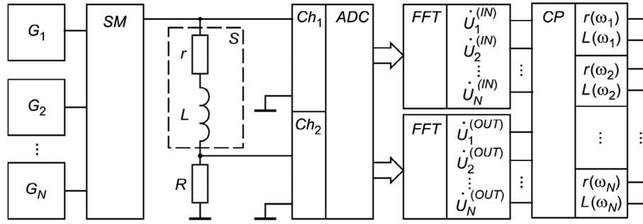
Fig. 1. Block diagram of the measuring device:  $G_1, G_2, \dots, G_N$  – blocks for specifying harmonic signals;  $SM$  – adder;  $S$  – parametric sensor;  $Ch_1, Ch_2$  – channels for digitizing input and output signals, respectively;  $ADC$  – analog-to-digital converter;  $FFT$  – discrete Fourier transform block;  $CP$  – computation unit.
