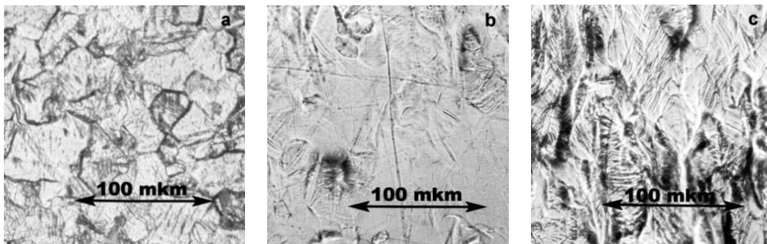
**FIGURE 3.** Ti alloy deformation structures. Strain  $\epsilon = 0.02$  (a),  $0.07$  (b),  $0.28$  (c)
