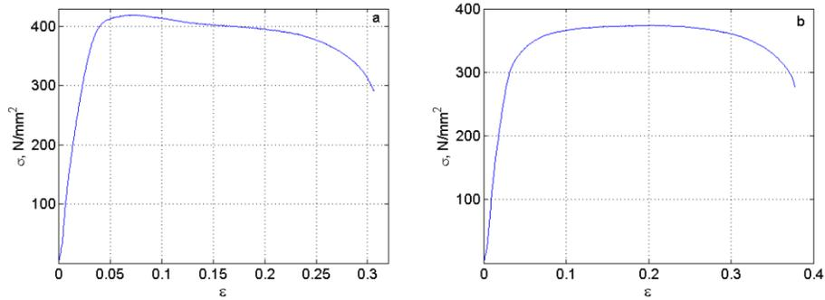
**FIGURE 1.** Strain hardening curves for Ti alloy specimens: (a) initial condition (unannealed), (b) annealed
