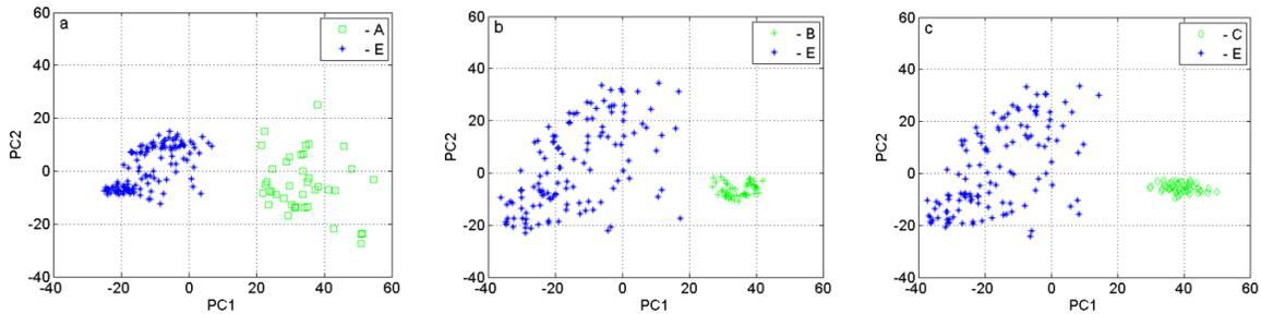
**FIGURE 4.** PCA analysis of AE peaks. Matching of the second AE peak of annealed specimens with the first (a), the second (b), and the third (c) AE peaks of unannealed Ti alloy specimens. Unannealed Ti alloy specimens: *A*—the first peak, *B*—the second peak, *C*—the third peak, annealed specimens: *E*—the second peak
