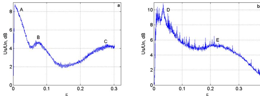
**FIGURE 2.** AE curves for unannealed (a) and annealed (b) Ti alloy specimens. Unannealed Ti alloy specimens: *A*—the first peak, *B*—the second peak, *C*—the third peak, annealed specimens: *D*—the first peak, *E*—the second peak
